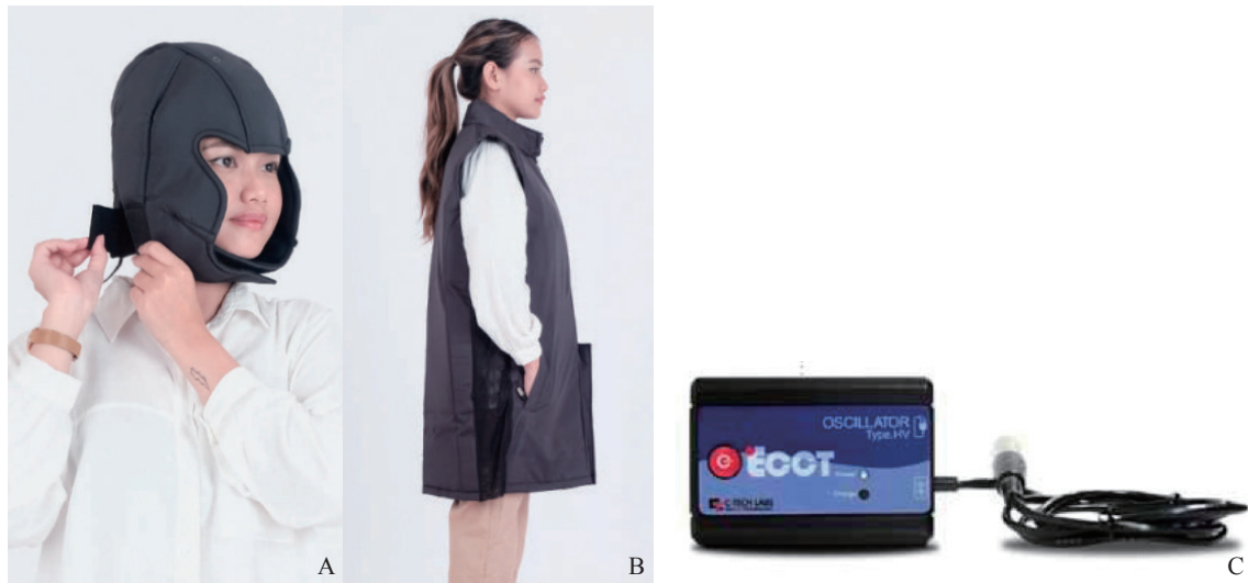
Fig. 2 The cord at the back connects to the battery along with the cord at the torso. This device is easy to put on and take off. A. Helmet type of ECCT device B. Truncal type of ECCT device C. ECCT oscillator
